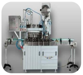
Air containing 21 % oxygen is detrimental to the stability and shelf life of beverages. The percentage of oxygen in the bottled product has to be reduced to a minimum since it is a risk for preservation of the bottled beverage. The vacuum pre-evacuation system ensures removal of oxygen during filling to give a packaged product of international standards.
